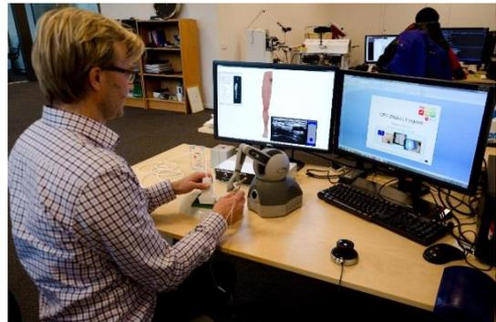
Fig. 1 The RASimAs training environment. The user interacts through the haptic devices with 3D patient specific models to perform a simulated RA operation [Photo courtesy of SenseGraphics<sup>2</sup>]
